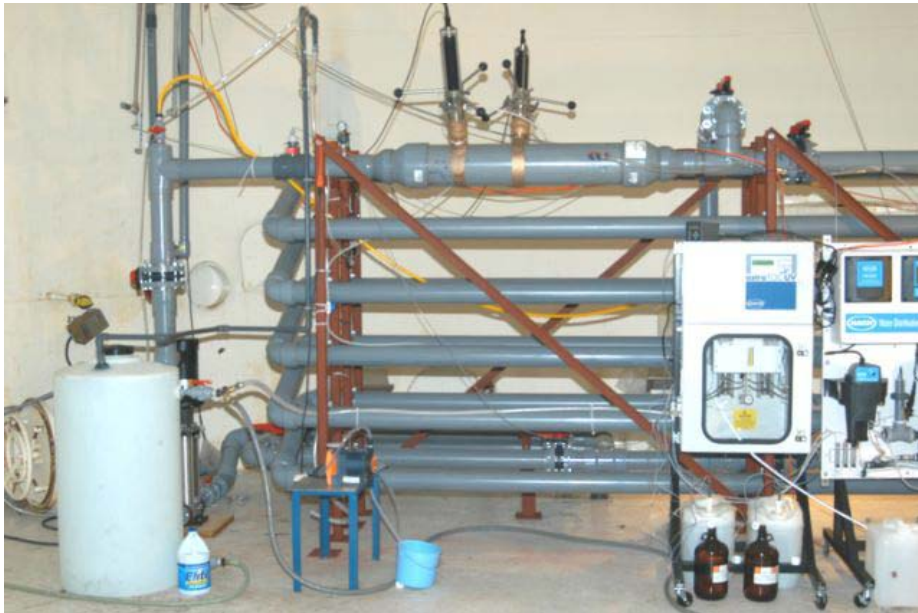
Fig 3. Flow loop testing verified transfer of fingerprints to a more realistic water sample scenario. Real-time loop tests were run on nicotine, ricin, anthrax and methanol.
