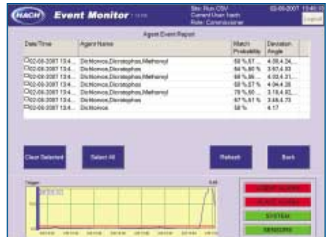
The trigger signal is compared to the agents housed in the Agent Library of the system and classifies the possible contaminant. This classification will help reduce the time it takes to identify the contaminant, possibly helping the team deploy the correct emergency response plan.
