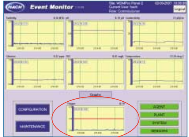
The trigger signal uniquely combines all 5 water quality parameters into one dimensionless vector signal. This signal is an indication of the overall health of the water in the distribution system.
