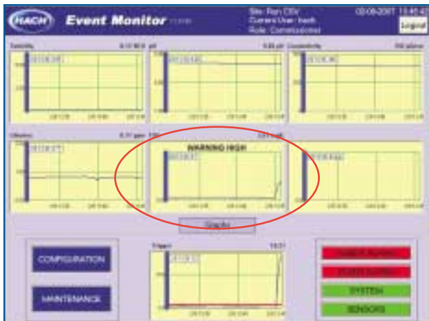
Trigger signal compares current water quality data to its baseline and once it "sees" a deviation from baseline, will alarm.
